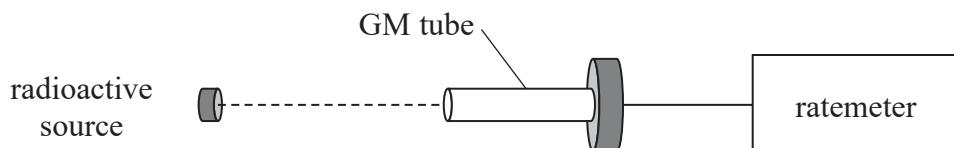
The ratemeter displays the count rate from all radiation detected by the GM tube.
