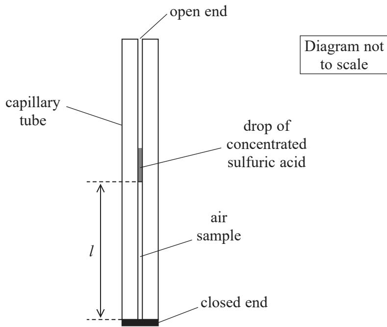
A sample of air is trapped inside the tube between the closed end and the drop of concentrated sulfuric acid.
